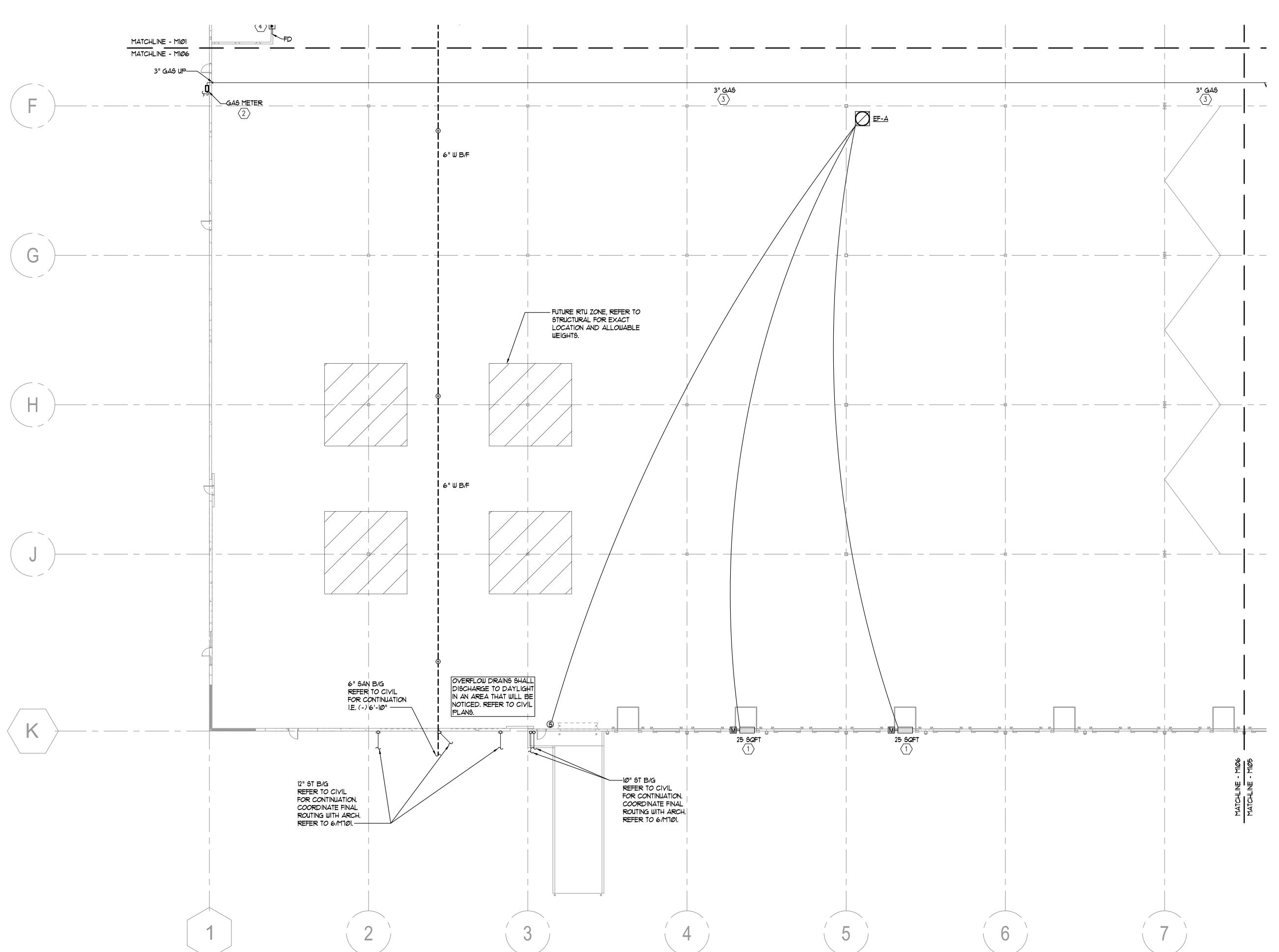
PROVIDE A STORM PROOF LOUVER WITH BIRD SCREEN WITH THE FREE AREA AS INDICATED. COORDINATE FINAL SIZING AND LOCATION WITH ARCHITECT. COORDINATE FINISH WITH ARCHITECT. PROVIDE WITH A SEPARATE MOD INTERLOCKED TO FAN AS SHOWN. MOD SHALL FULLY OPEN PRIOR TO FAN ENERGIZING. LOUVERS SHALL BE GREENHECK EHH-501X, HURRICANE RATED FOR MISSILE IMPACT, 200PSF, AND WIND DRIVEN RAIN RATED WITH WELDED CONSTRUCTION, OR APPROVED EQUAL.
