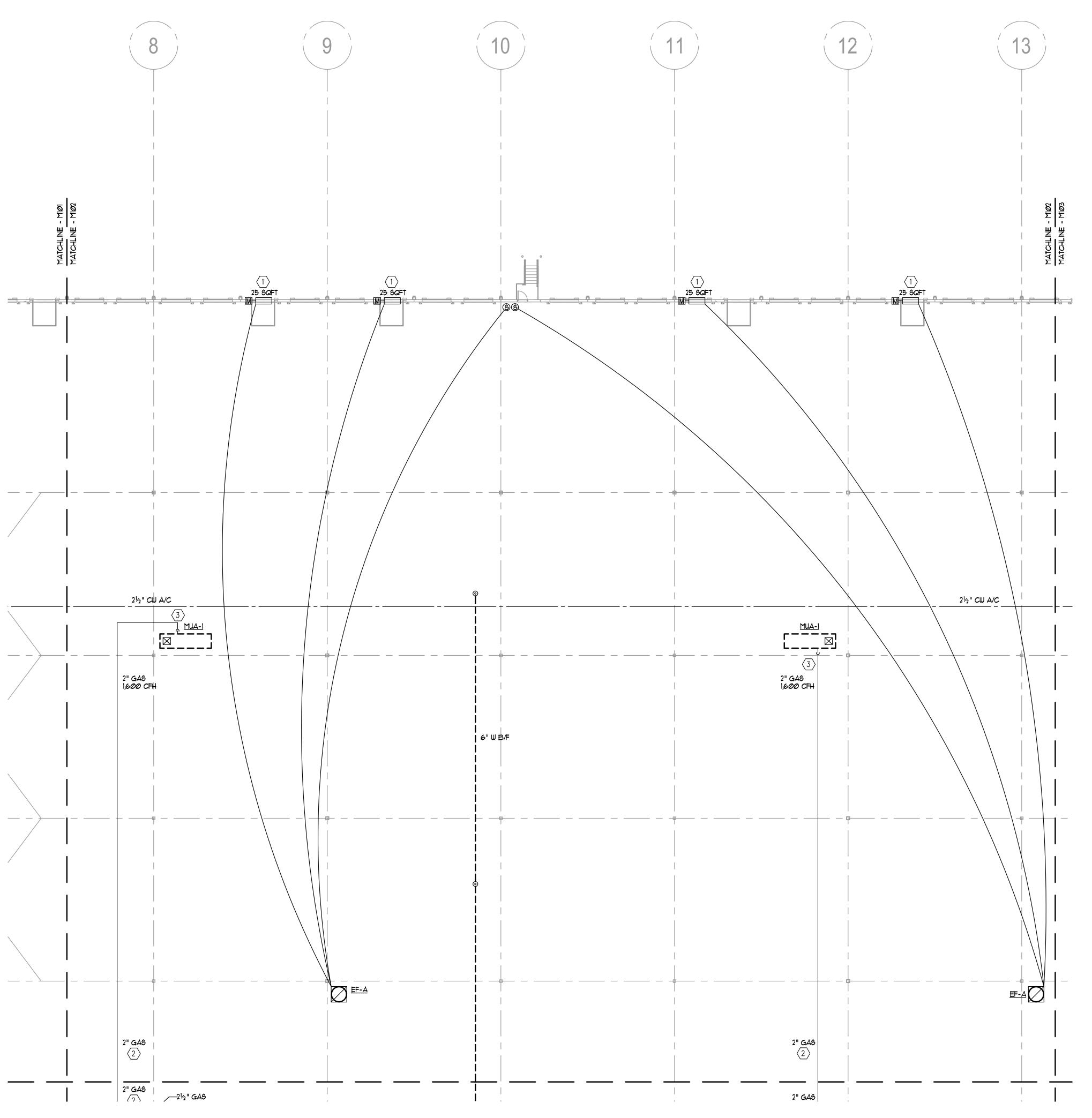
PROVIDE A STORM PROOF LOUVER WITH BIRD SCREEN WITH THE FREE AREA AS INDICATED. COORDINATE FINAL SIZING AND LOCATION WITH ARCHITECT. COORDINATE FINISH WITH
